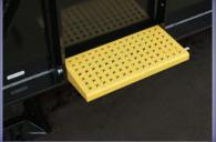
Convenient fold-down step and grab handle located on both sides of the trailer are standard equipment
